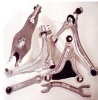
Figure 2. Raufoss Technology AS is an innovative company that designs and produces automotive components in aluminium. The studied control arm is produced according to the patented ExtruForm® process.
